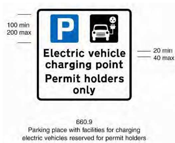
Figure 3 Electric Vehicle Signage
